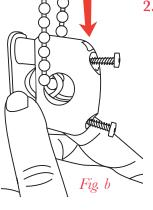
**2.** Insert a 2" screw into each hole, then position the device on the wall or moulding, pulling down slightly to ensure proper tension (*fig. b*). The chain should be taut on both sides.
