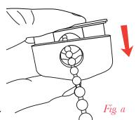
**1.** Compress the tension device and slide it all the way down the chain (fig a).
